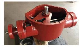
To ensure leak free seating, all RCV series are equipped with a lift turn lower type gearbox. The gearbox is designed to lift the valve out of the seat before rotating open and to lower the plug into the seat as it is closing. This prevents rubbing of the metal seats extending their life, providing a leak free seal, and reducing operating torque.
